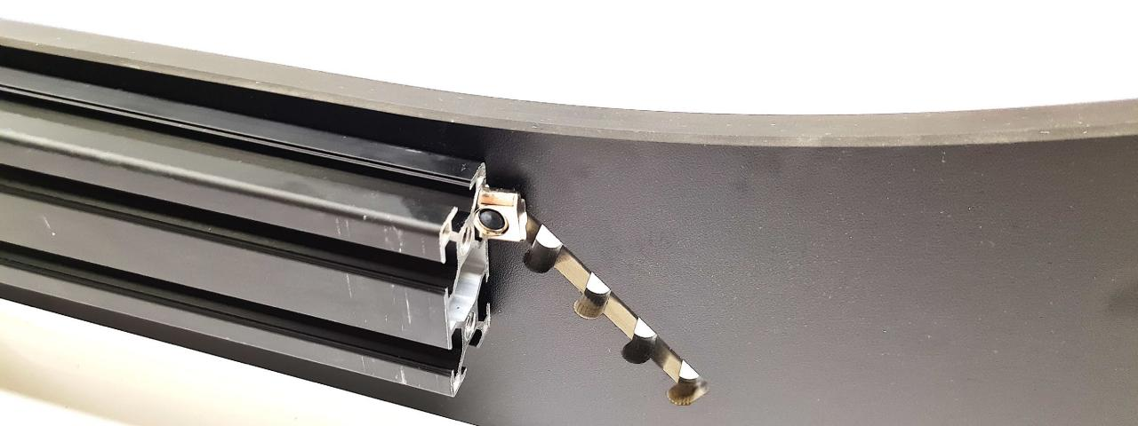
Slide the T-nuts in the slots like shown in the picture. Start from rear to front.
