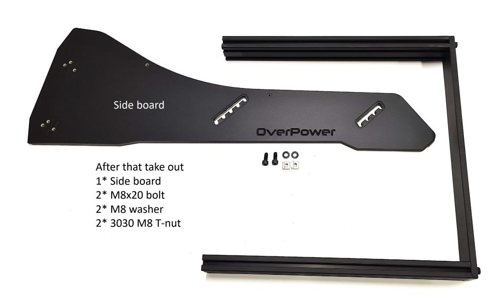
Attach the bolts and T-nuts to the side boards like shown in the picture. Do not tighten them yet.
