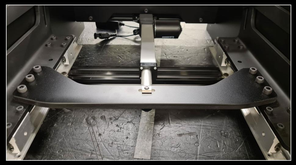
Attach the actuator to the cross support with the slide and bolt from the previous phase
